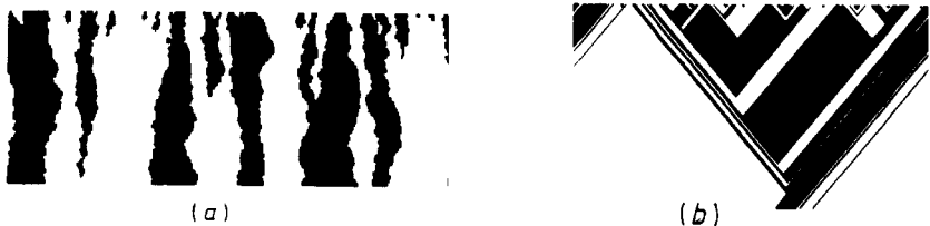
Figure 1. Evolution of the (a) Glauber CA and (b) Metropolis CA from random initial configuration through the first 50 time steps. Horizontal axis: space coordinate, vertical axis: time, increasing downwards. Black regions: s_i = +1 ; white regions: s_i = -1 .
